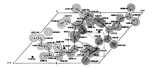
Fig.1 Composite electron density distribution viewed along the <u>b</u>-axis. Contours are drawn at intervals of 2 e.Å<sup>-3</sup> beginning at 2 e.Å<sup>-3</sup>; those for the bromide and chloride ions are not drawn. A part of the map is shown separately. The fractional  $\chi$ -coordinate is given after the name of the atom.
